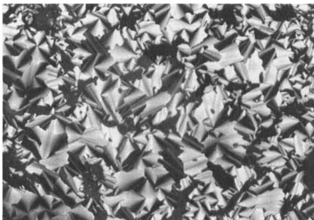
Figure 3. Liquid-crystalline texture shown by CuP7 at 165°C; crossed polarizers.
